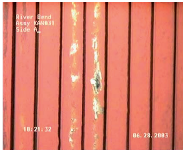
FIG. 5.22. Failure location noted from bubbles escaping at a defect in a peripheral rod [5.43].
