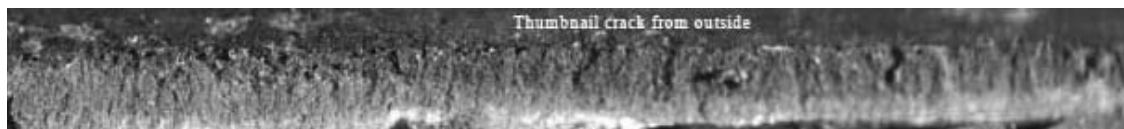
FIG. 5.47. Photo of crack (dark region) which started from the outside after the power ramp of a high burnup rod, (20X).
