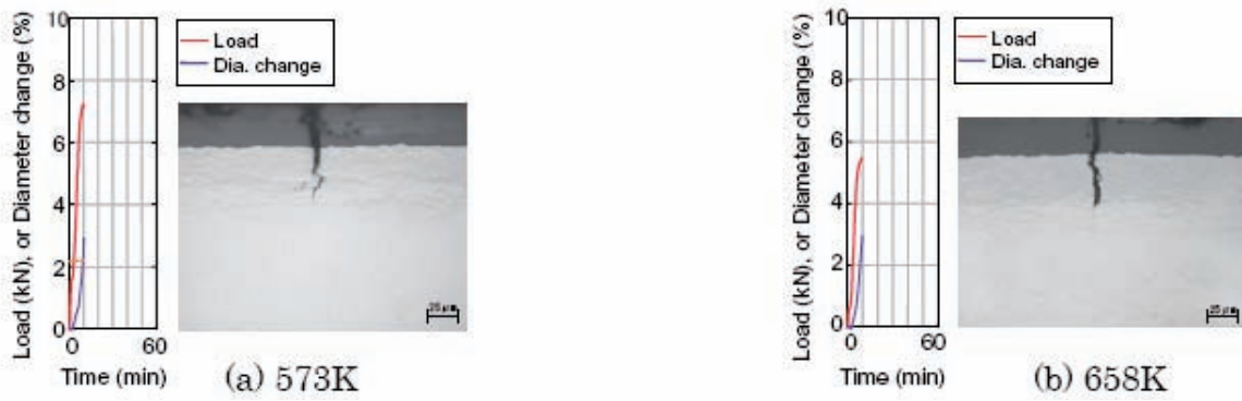
FIG. 5.52. Incipient crack formation through an EDC crack propagation test with no holding period.
